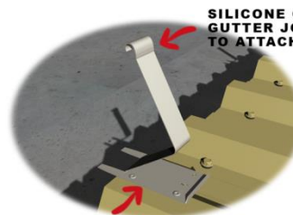
ATTACH BRACKETS TO CLADDING WITH POP RIVETS
