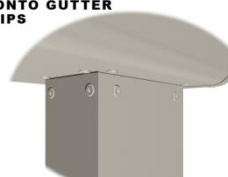
ATTACH STOP ENDS AND DOWNPIPE NOZZLE WITH SILICONE & RIVETS
