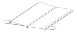
Note that the different cover width versions of AvantaLine™ cladding can be used together to create different architectural appearances
