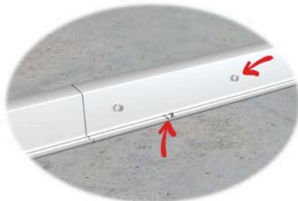
MEASURE & MARK POSITION OF INTERMEDIATE PORTAL FRAMES
