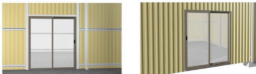
SIDE WALL GLASS SLIDING DOOR IN PLACE
