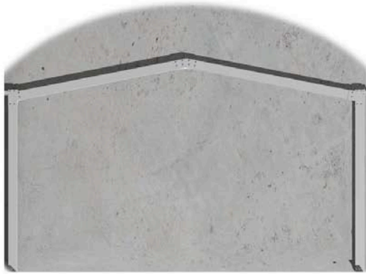
ASSEMBLE PORTAL FRAME ON THE GROUND
