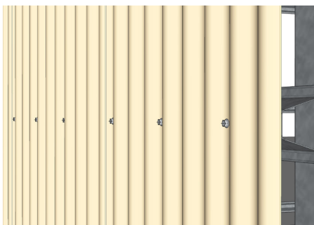
Screws as per wall sheeting profile
